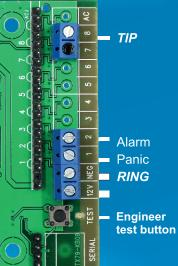
A simple two wire installation allows extra data to be sent in the Contact ID format. Open/lock-up by user number or alarm by partition and zone can be sent in a single signal.
