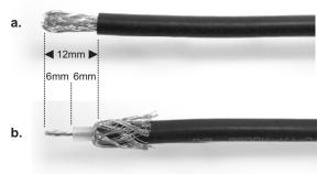
Fray and pull back the braiding and strip off 6mm of the inner white insulation leaving 6mm of the inner wire exposed.
